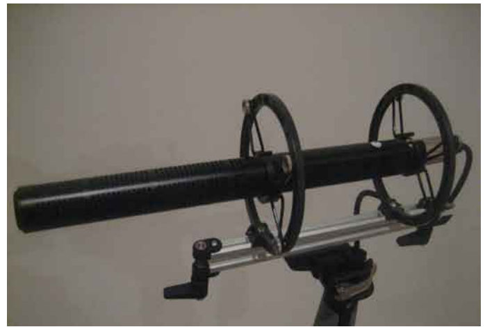
Figure 4. Microphone shock mount setup The microphone is suspended by elastic bands that reduce movement sound by absorbing vibrations.
