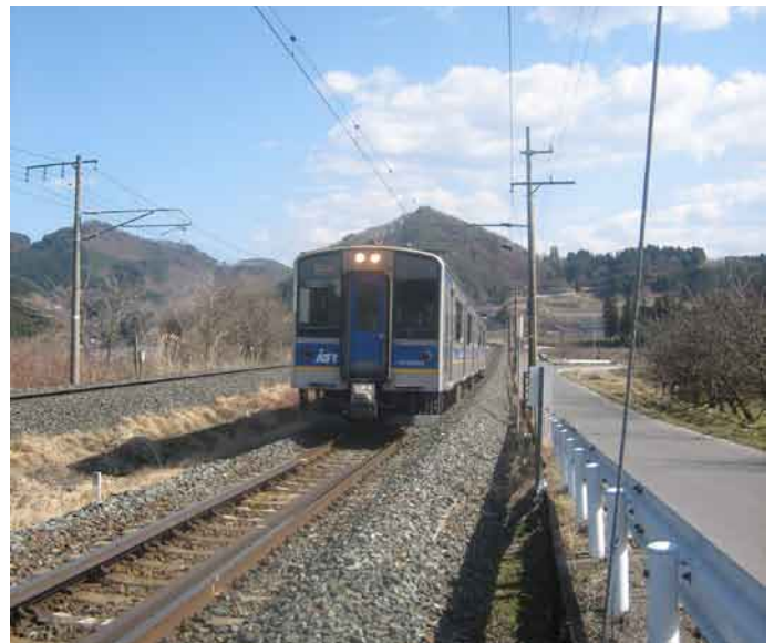
Figure 9. Fast moving object at close proximity The wind rush from this train made the recording unusable.
