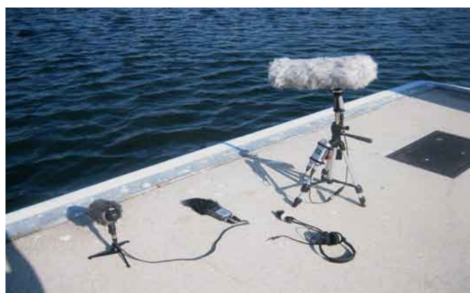
Figure 5. Multiple microphones used to record an event Using a series of microphones in different positions set to different input levels increases the chances of capturing good samples of events with very high volume levels, or just to capture a different point of view.
