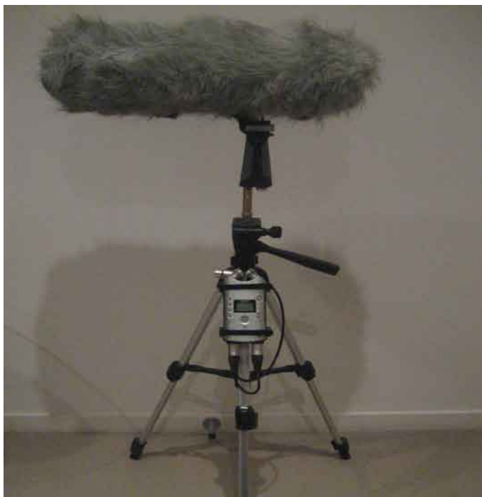
Figure 3. Mounted Microphone setup A traditional microphone stand is fairly heavy, but a camera tripod can be a good lightweight compact solution for reducing vibration and allowing hands free operation.
